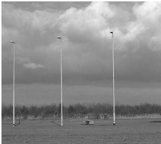
Fig. 2. Experimental lighting columns at the SRI test site.
