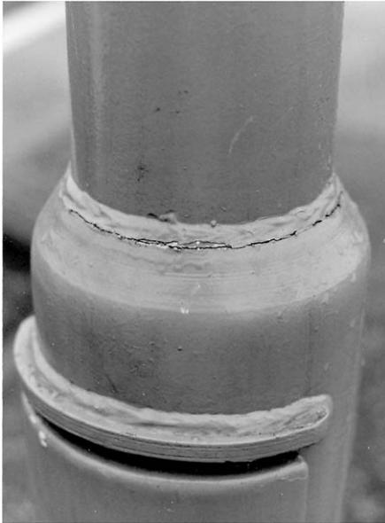
Fig. 1. Fatigue crack in a lighting column in service.
