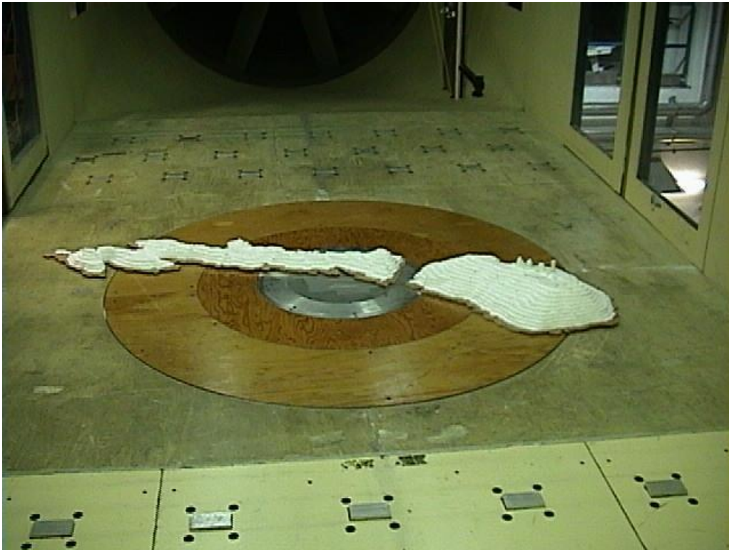
Figure 2. Model of Waglan Island used to determine anemometer corrections in the wind tunnel of the Hong Kong University of Science and Technology
