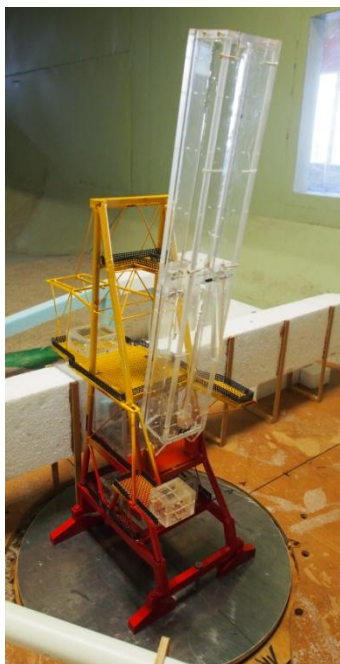
Fig. 5 1/80 scale wind-tunnel model of a shiploader (Structure C)
